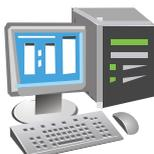
**Host Computer & Software:** The host computer or server contains the central database of cardholders, permissions, and the system software needed for set up and operation. Software typically provides badging, scheduling, monitoring and reporting.
